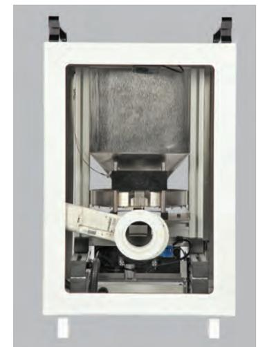
NHP access perspective. NHPs reach through the RFID reader tube to access metered food, or present RFID chips to access individually restricted diets.
